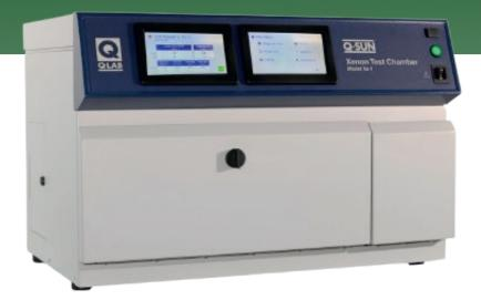
Samples of the material are then placed in the weatherometer and exposed to a controlled cycle of light, humidity, and temperature.
